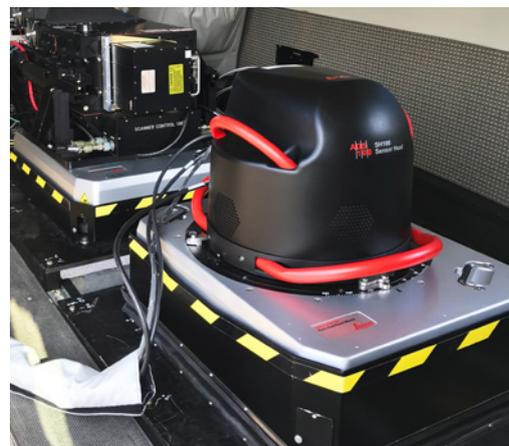
Leica PAV100 aircraft installation
